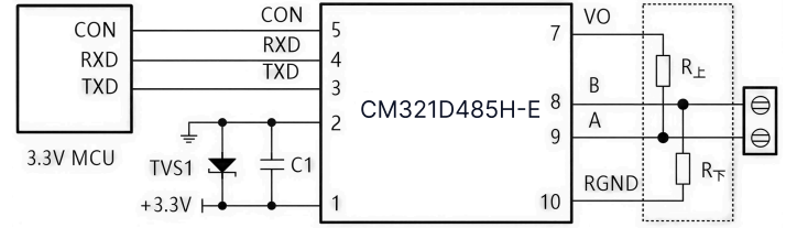
Fig 4. MCU 3.3V Power Supply Application Circuit
